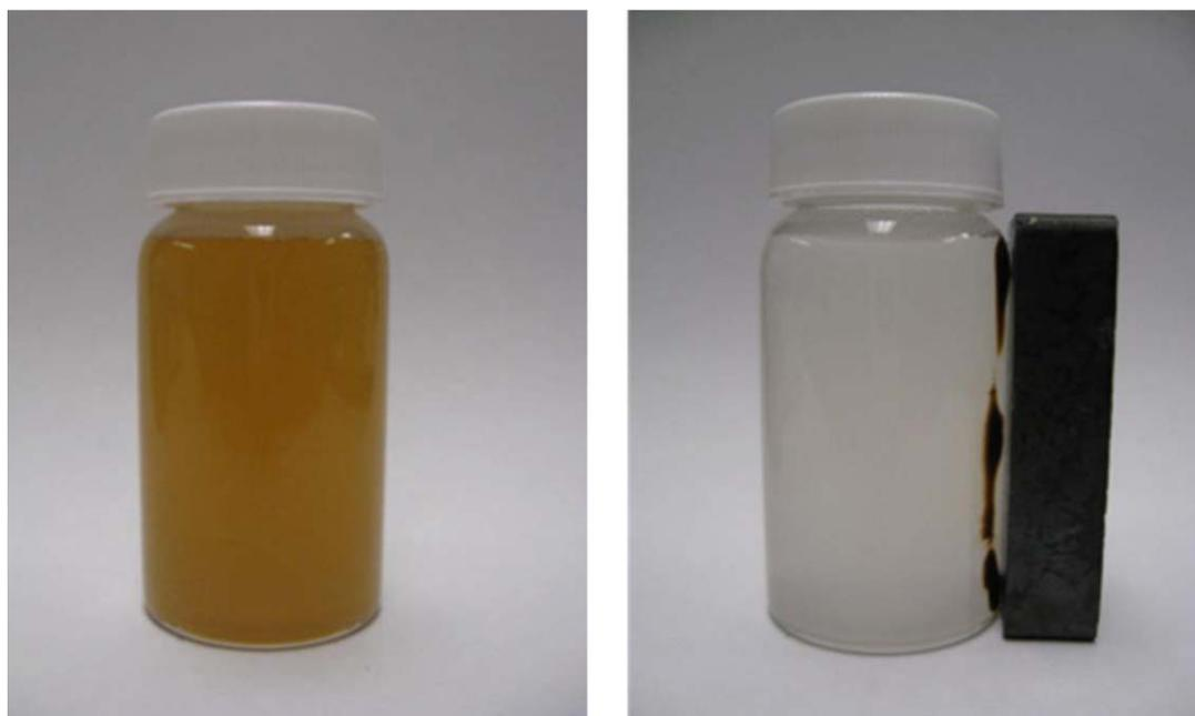
**Figure 5.** Migration of PLA-hydrophilic IONPs composite particles under the magnetic field by a magnet; before (left) and after (right). [Color figure can be viewed in the online issue, which is available at [wileyonlinelibrary.com](http://wileyonlinelibrary.com).]
